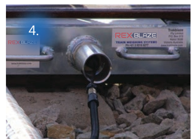
4. Connecting the cables, wireless option also available
